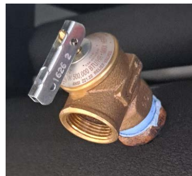
Figure 1. Cash Acme FWL-2 pressure relief valve installed on copper pipe near electric heating element
