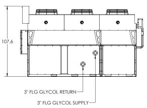
\*APPROXIMATE DIMENSIONS - DO NOT USE FOR PRE-FABRICATION OF CONNECTING PIPING
